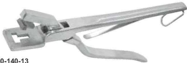
40-140-13 Ear Notcher S.S. Design in the Center of the ear
